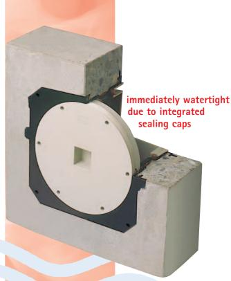
Due to the integration of a gas- and presswater-tight sealing cap systems BKD and KD (KD 85, KD 150) offer a protection against pressing water immediately after installation. The interior of the bushing stays clean during concrete works and there are no additional costs for blind plugs on spare bushings. Accessory tools like system or square wrenches facilitate efficient removal.
