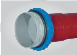
System connection D (for BKD 150) for gas- and watertight connection to a bayonet sealing collar. Available for system: KSS B150.
