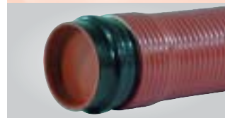
Plug-type Sleeve SM for connection of a smooth-walled cable protection tube. SM 110 , e.g. for smooth-walled tubes with an outside dia. of 110 mm. Available for systems: KSS B150, KSS 150, KSS 110, KSS 85, SM 75 , e.g. for smooth-walled tubes with an outside dia. of 75 mm. Available for system: KSS 85
